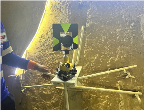
Figure 1 Reference Monument mounted on bracket attached to Tunnel's wall
