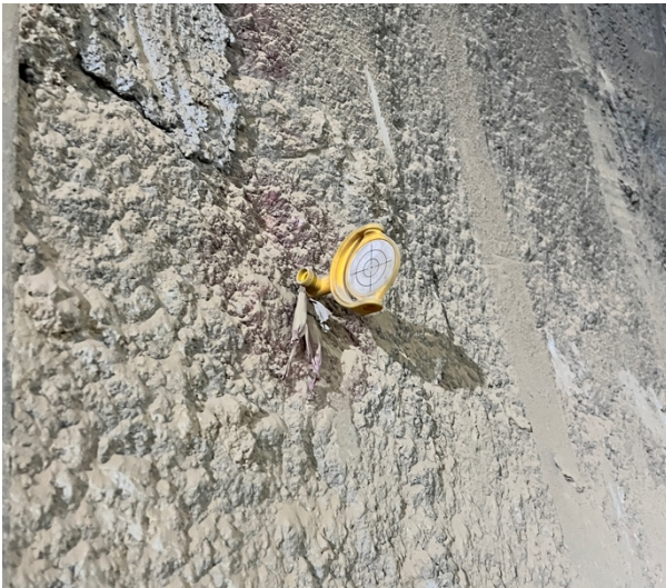
Figure 2 Target for Convergence Monitoring by conventional method
